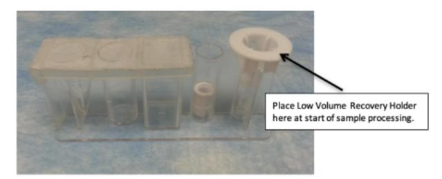
11. If using the Microfuge tube, add 300µL of Binding Buffer to the Microfuge tube in the sample retrieval position on the cartridge (well No. 5) as showing below.
